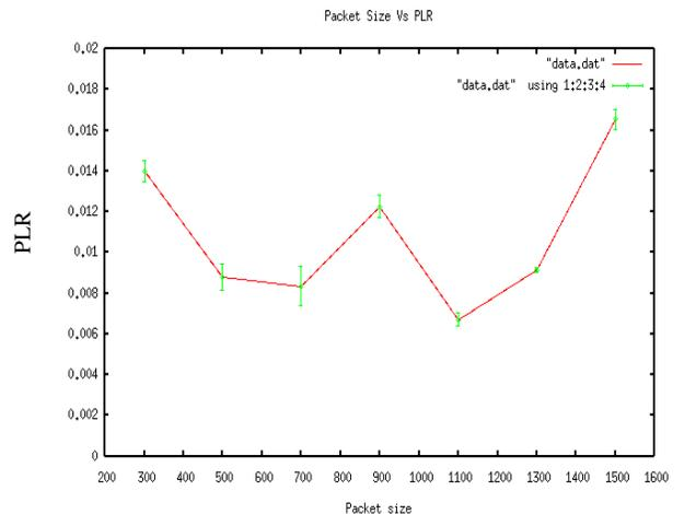
Figure 4.3 PLR Vs Packet size
